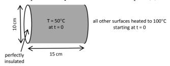
$$\rho = 7820 \; kg/m^3 \qquad \frac{properties \; of \; steel}{C_p = 461 \; J/(kg \; K)} \qquad \quad k = 23 \; W/(m \; K)$$
